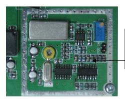
Test point frequency lock signal for model: PLL-11031K only
