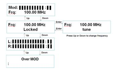
The PLL of transmitter will tune. After the PLL is locked to the frequency, LED will be displayed on LCD panel.
